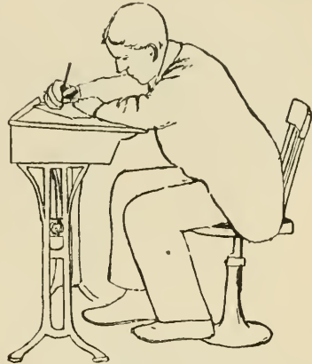
FIG. 43. — Illustrating too great a space between the seat and desk, causing pupil to stoop too much, inducing round shoulders.
